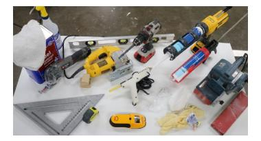
Level, Circular Saw (minimum 48 tooth carbide saw blade), Tape Measure, Drill, Heavy Duty Caulking Gun, Square, Router / Jigsaw (fine tooth blade), Grinder with appropriate blade to remove substrate or Tiger Saw with appropriate blade to remove substrate, Denatured Alcohol, Clean White Rags, Wilsonart Complete Color Matched Sealant, Safety Glasses, Hearing Protection, Protective Gloves, Protective Footwear, Dust
